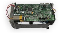
The state-of-the-art IR-400 Series NDIR Optical Benches from Infrared Industries are designed to do highly accurate gas analysis and to meet worldwide gas measurement standards. Selectivity of specific gases is obtained via an optical interference filter. Components are easy to reach and replace, which makes the unit highly serviceable.
